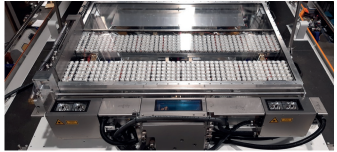
CIS with open lid showing the individual sensors: CRS (middle bottom), two LPS (left and right bottom), and LED panels for illumination. The cameras for wire wear measurement are located between the LED panels (not visible). The metal rails are used for the semi-automatic cleaning system.
