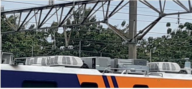
CIS installed on a train: The system is located between the two white air conditioning modules.
